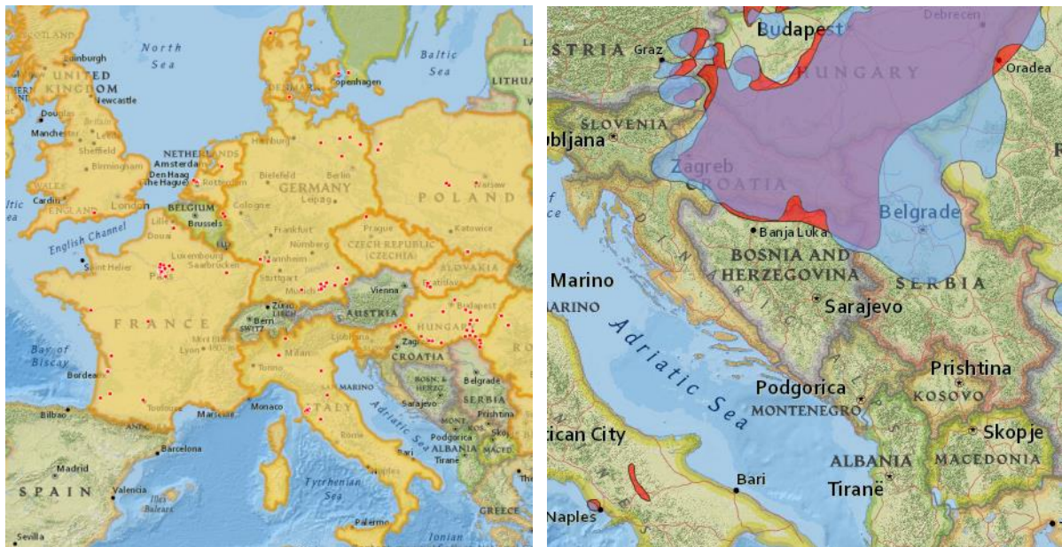
Figure 30: Maps showing existing district heating systems (red dots) with geothermal energy (left) and potential for geothermal energy (right); Legend: temperature > 50°C at 1,000 m depth (blue) and temperature distribution > 90°C at 2,000 m depth (red); purple colour = overlap of the two layers. (Sources: http://map.mfi.hu/geo_DH/ )
