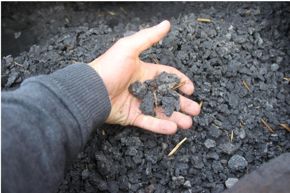
Figure 18: Molten bottom ash after straw combustion (Source: Rutz D.)
