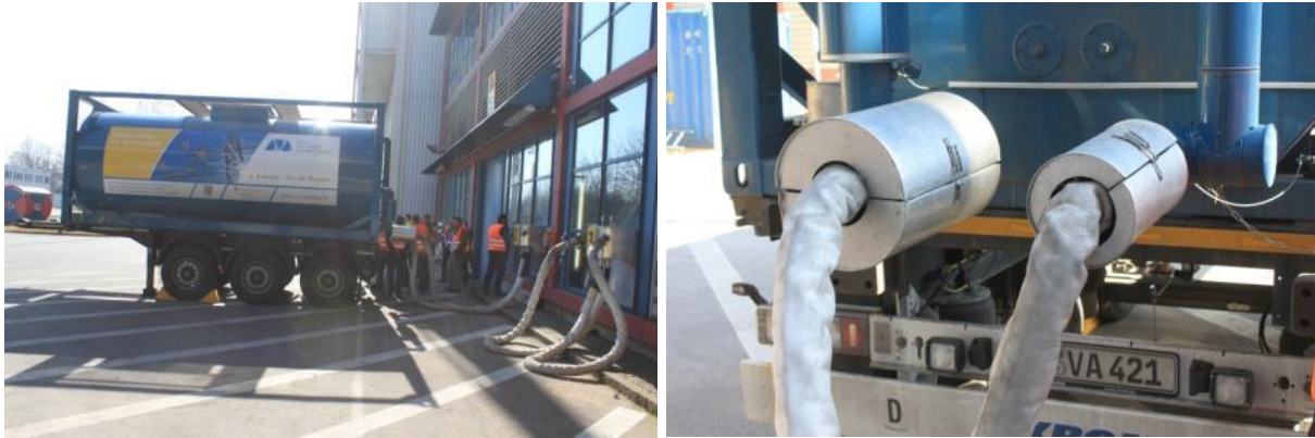
Figure 42: Heat storage container on a trailer at a waste incineration plant (Augsburg, Germany) (Source: Rutz D.)
