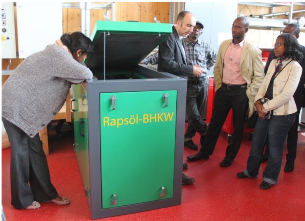
Figure 28 Rapeseed oil CHP unit (Source: Rutz D.)
