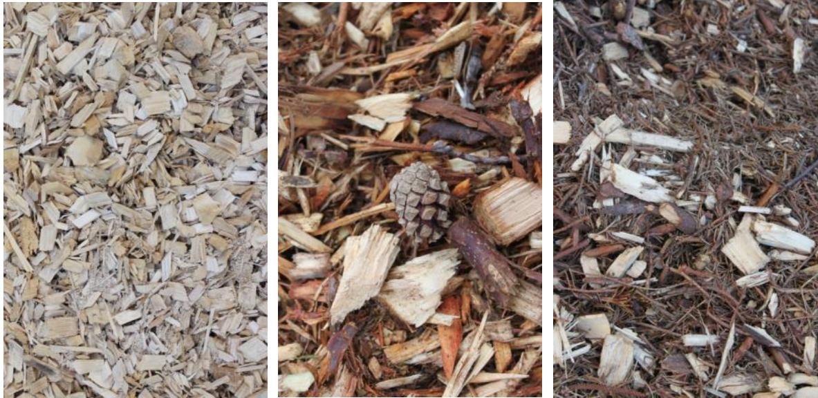
Figure 14: High quality (left) and low quality (middle, right) woodchips in Germany (Source: Rutz D.)
