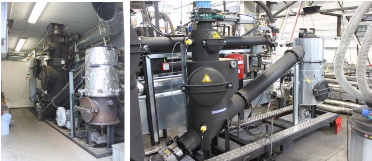
Figure 21: Small-scale gasifiers in a container (left) and during manufacturing (right) of the company „SpannerRE“ (Source: Rutz D.)
