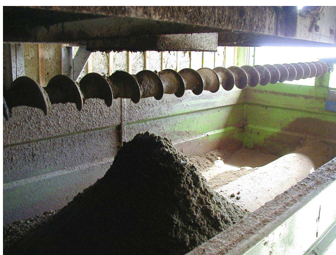
Figure 6.5 Fibers collection wagon, with distribution screw (ANGELIDAKI 2004)
