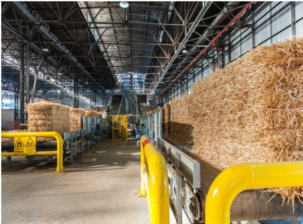
Figure 11: Biomass fed in the conveyor system
