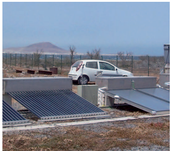
↑ TECHNOLOGY: MULTI EFFECT SOLAR BASINS ENERGY SOURCE: SOLAR THERMAL ENERGY WATER SOURCE: BRACKISH WATER DAILY CAPACITY (NOMINAL): 15-18 LITER/M 2 YEAR OF INSTALLATION: 2005 TYPE OF INSTALLATION: R&D LOCATION: GRAN CANARIA INSTALLED BY: SOLAR-INSTITUT JÜLICH
